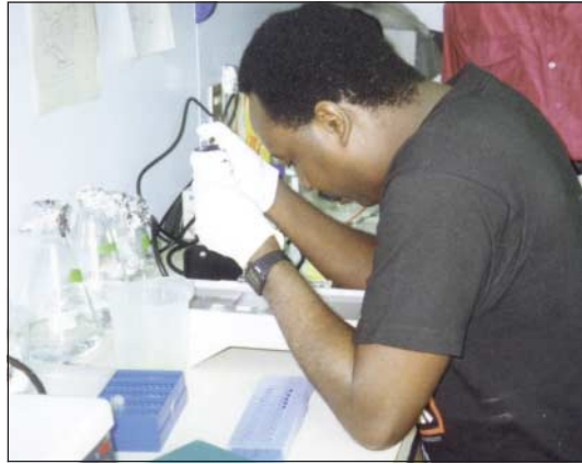
Fig 2 Loading DNA samples for electrophoresis using Parafilm on a makeshift rack to remove mineral oil after polymerase chain reaction
